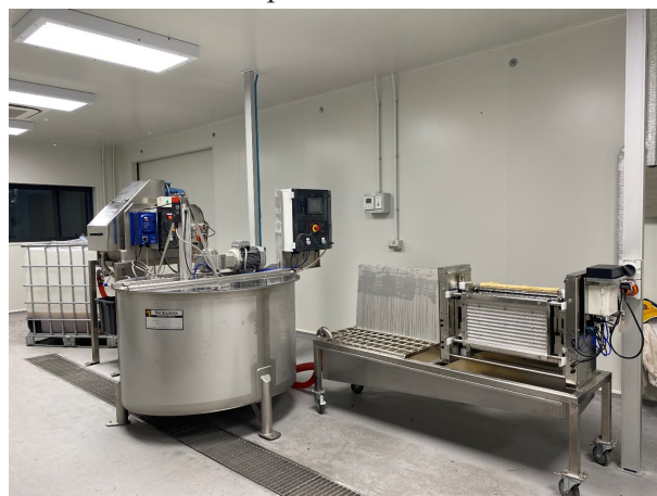
Figure 3. The Extraction Room houses the NZ Boutelje compact extraction system including a loosener for frame processing, 24 frame extractor; honey and wax centrifuges allowing honey to be pumped straight into a bulk container.
