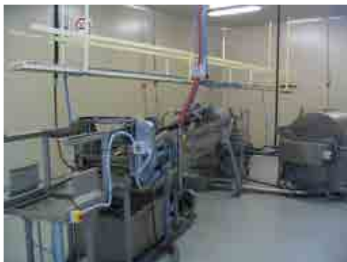
Twin Beequip 72 frame HR extractors fed by a Beequip chain feed uncapping machine, B-QUAL accredited premises
