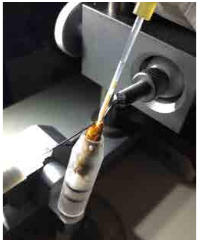
Close up of the Schley instrument and a virgin queen pre-insemination. The virgin is held in place and given a steady, low dose of CO2 during the procedure. Her vaginal orifice is held open using a ventral hook and sting forceps.
